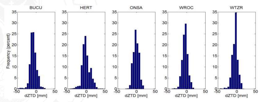
An optimal solutions among all stations were obtained for 2mm/h to 5mm/hour random walk. The results were slightly biased: -4 mm to +7 mm (note: DD vs PPP solution) and the standard deviations varies from 7 mm to 12 mm.
